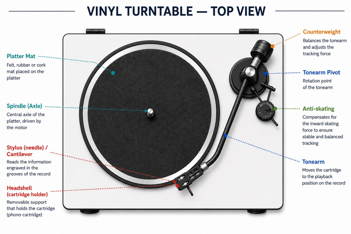
Figure 1 — Simplified anatomy of a vinyl turntable
